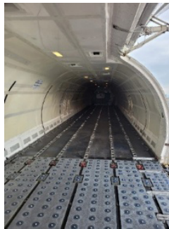
Figure 2: The roller floor inside the aircraft.
