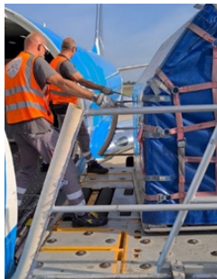
Figure 3: Two of the acquired workers involved in the loading of the ULD from the ACL inside the airplane.
