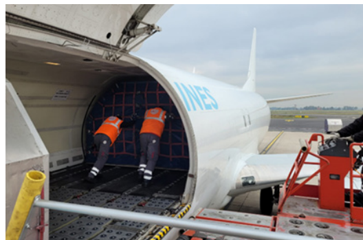
Figure 4: Two of the acquired workers involved in the task of pushing the ULD on the roller floor inside the airplane.
