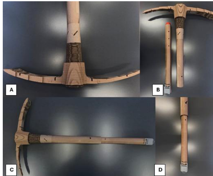
Figure 3: Cardboard mock-up showing the tool structure and mechanism (A), dual-ended head dimensions—pick and flat blade (B), detachable telescopic handle (C), assembled tool (D), and light position on the front face of the handle.
