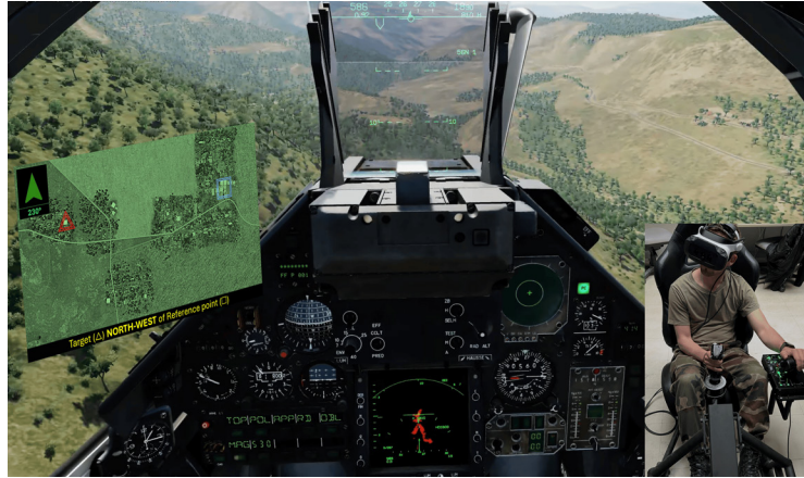
Figure 1: Immersive flight simulation environment. View from the virtual cockpit during the low-altitude terrain-following flight, with the target-validation display integrated into the cockpit.
