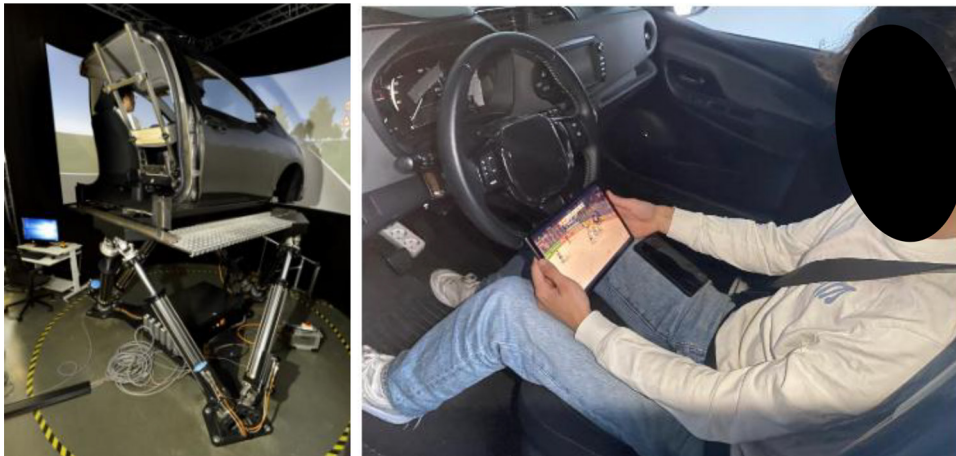
Figure 1: (left) Delft Advanced Vehicle Simulator (DAVSi) (right) participants' posture while being driven in the experiment.
