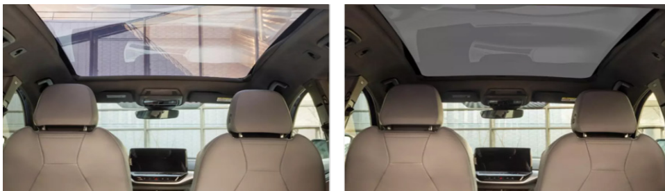
Figure 2: Saint-Gobain Sekurit AmpliSky Ombra, clear (left) and opaque (right) state (Saint-Gobain, 2026).
