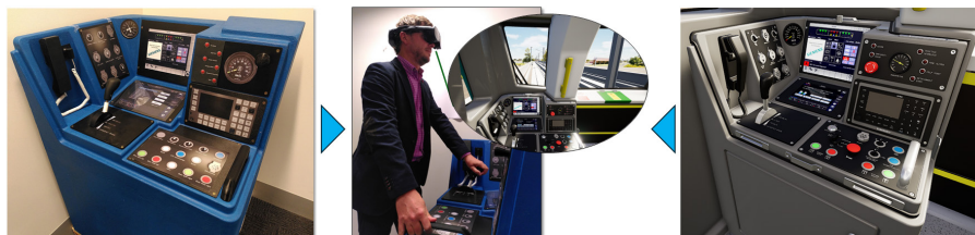
Figure 3: Illustration of how physical (left) and virtual (right) models enable multimodal experience operating the DMI (middle).
