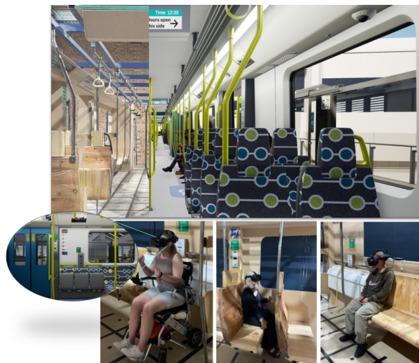
Figure 4: Passenger Saloon of physical (upper left) and virtual (upper right) models, when fused (lower row), enable multimodal, ecologically valid passenger testing experience.
