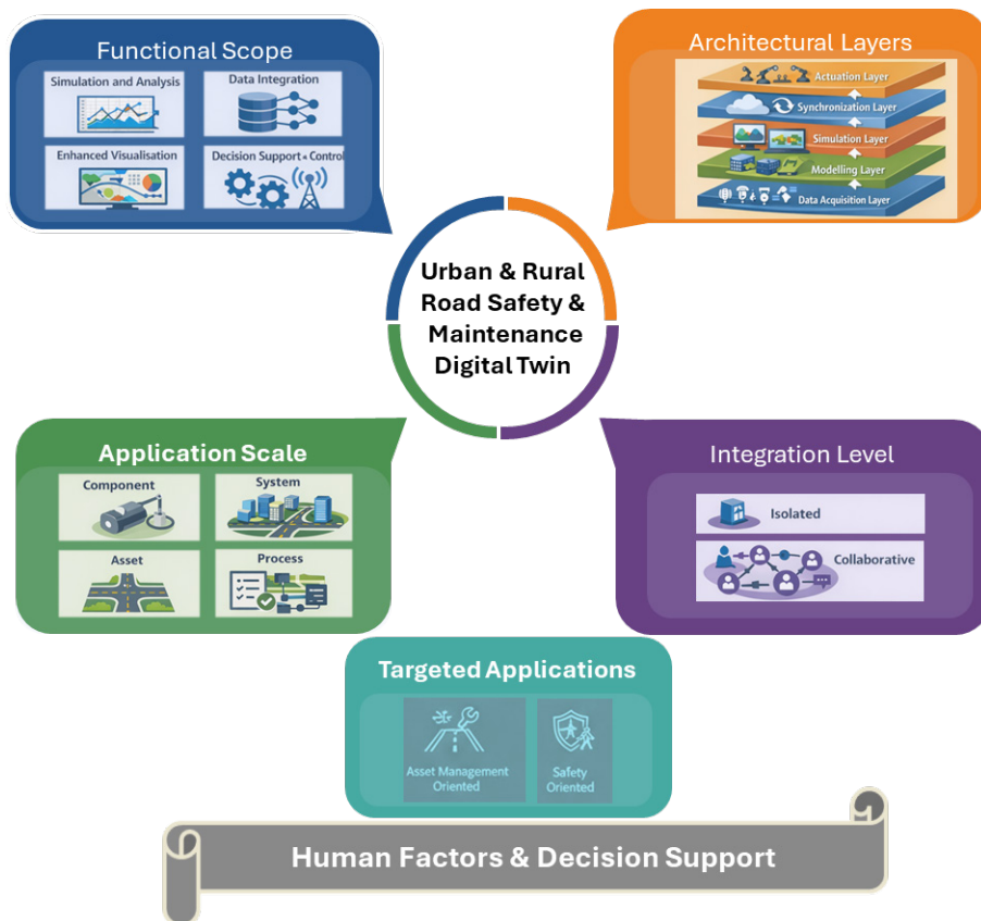
Figure 1: Proposed digital twin taxonomy for urban and rural road safety and maintenance applications.
