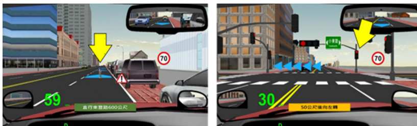
Figure 2: Simulation of an AR-HUD system providing dynamic navigation and safety alerts based on real-world road events. The left panel illustrates the system's response to a pedestrian (indicated by the yellow arrow for reference), triggering a red exclamation warning icon on that pedestrian spot, alongside a green straight-ahead navigation banner. The right panel demonstrates the system identifying an upcoming red light (indicated by the yellow arrow), replicating the signal status on the traffic light location, and updating the navigation banner to a yellow left-turn alert. For the turn feature, the AR-HUD projects a series of blue directional arrows directly onto the road surface to guide the vehicle's path, while simultaneously providing telemetry such as the current speed in green (e.g., 30, 59 KPH) and the 70 KPH speed limit.
