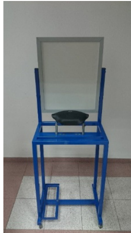
Figure 3: SRS system pyrotechnics firing station.
