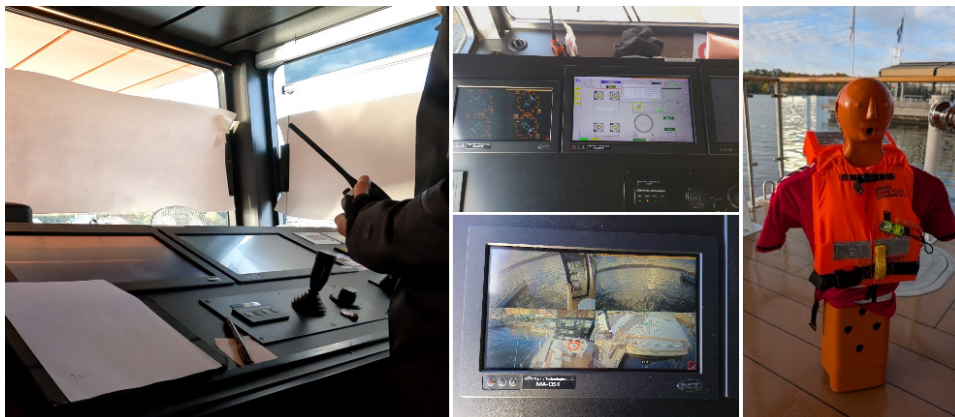
Figure 2: Left: ROC setup. Middle: Thruster control panel (top), video feed panel (bottom). Right: MOB dummy.
