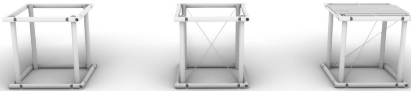
Figure 4: From left to right: Bamboo FlexGrid base frame, reinforced module, and functional seat surface.
