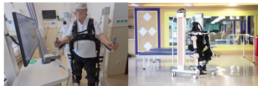
Figure 2: BCI-controlled lower-limb exoskeleton and treatment scenario (Adapted from RoboCT, 2026).
