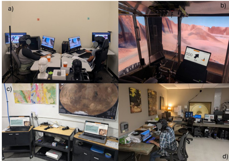
Figure 1: Research environments where the MIND software has been deployed. a) Depicts a traditional lab environment with a monitor, keyboard and mouse. b) Depicts a Mars rover simulator with surround TV screens, laptops, and a joystick. c) Depicts the work stations at the Mars Desert Research Station in Hanksville, Utah. d) Depicts the fMRI set up with a participant in the control room and the other participant in the scanner.
