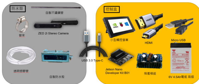
Figure 2: Hardware architecture of the underwater stereo camera system, including the stereo camera, embedded device, and communication module for continuous data acquisition and cloud-based processing.
