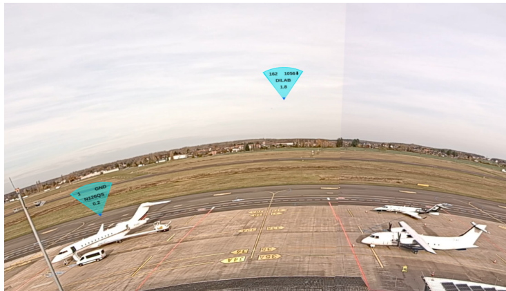
Figure 1: BWE Airport view inside the virtual tower app with labels. Label dimension decreases with distance, with speed and altitude disappearing over 5nm.
