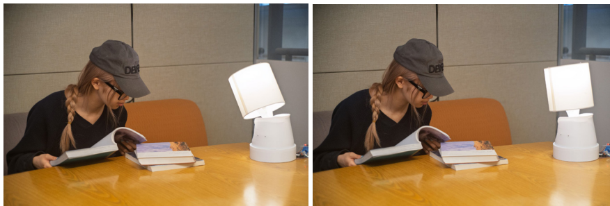
Figure 2: The user and the lamp are in the same reading environment. The lamp is tracking the user's behavior and providing physical feedback.
