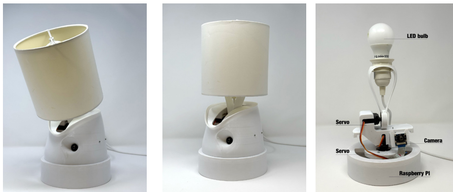
Figure 1: Lamp in receptive mode, lamp in attention mode, and a labelled image of the components.
