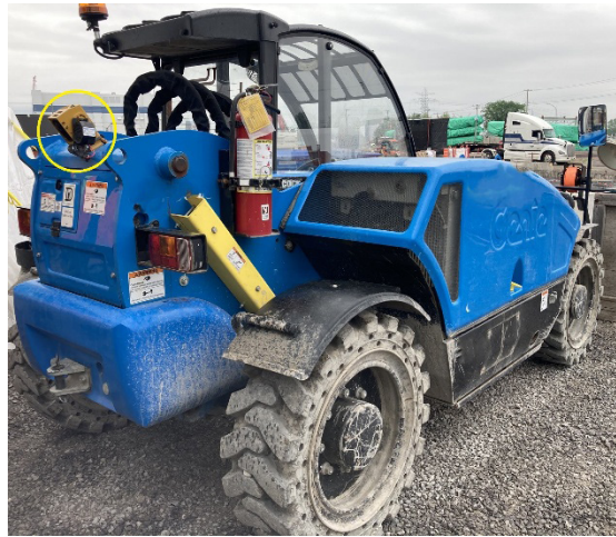
Figure 1: PDDs (artificial intelligence enhanced camera) installed on the rear of a telehandler used on a construction site.
