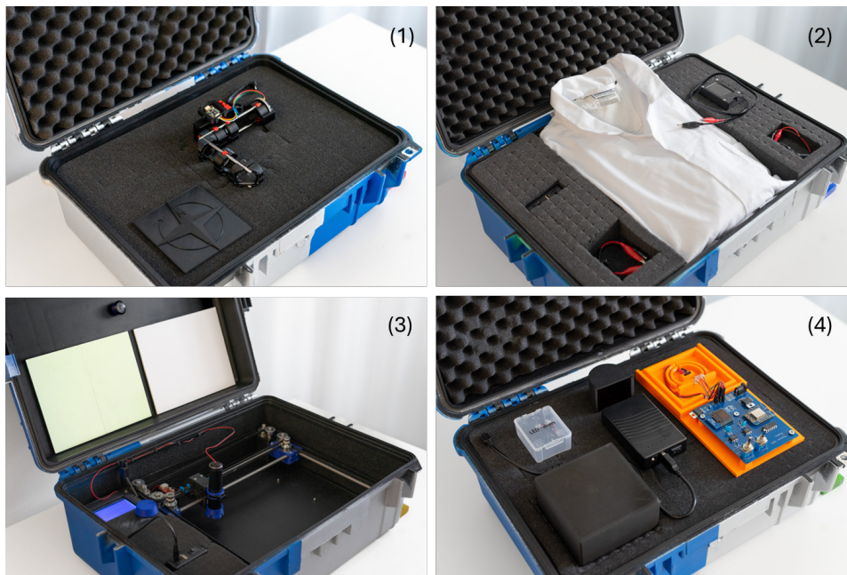
Figure 1: Overview of the four puzzle boxes. (1) AR magnetometer display for geomagnetic field-line visualisation. (2) Laboratory coats with sewn-in LED matrices and low-voltage circuit. (3) CNC-driven UV lamp with phosphorescent element. (4) NV-diamond magnetometry setup.
