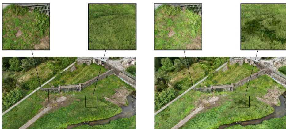
Figure 3: Reconstruction of a scanned area: our method on the left, baseline on the right. In the zoom-ins, we can observe areas that are too bright in the baseline, and correctly reconstructed with enough detail by our method, as well as spurious dark patches in the grass visible only in the baseline.
