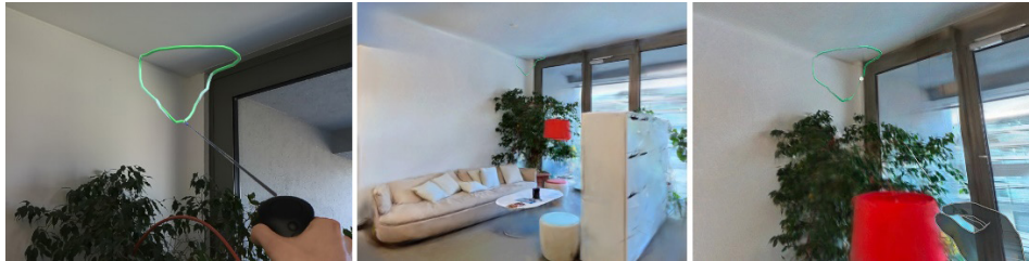
Figure 4: Overview over the annotation and reconstruction process. The left image shows the user's view through the Magic Leap 2 device with a set label. The center image shows the reconstructed scene within the Unity3D editor. The right image shows a first-person view through the VR glasses where the user sees the set labels in the reconstructed scene.
