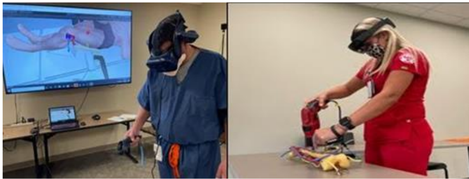
Figure 1 b: (left) : Interacting with a VR environment; (right): interacting with a MR environment (user can see/interact with VR scene and physical world simultaneously)
